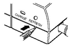
The REFRESH light blinks during the discharge process. This process takes about 10 hours.  $\,$
